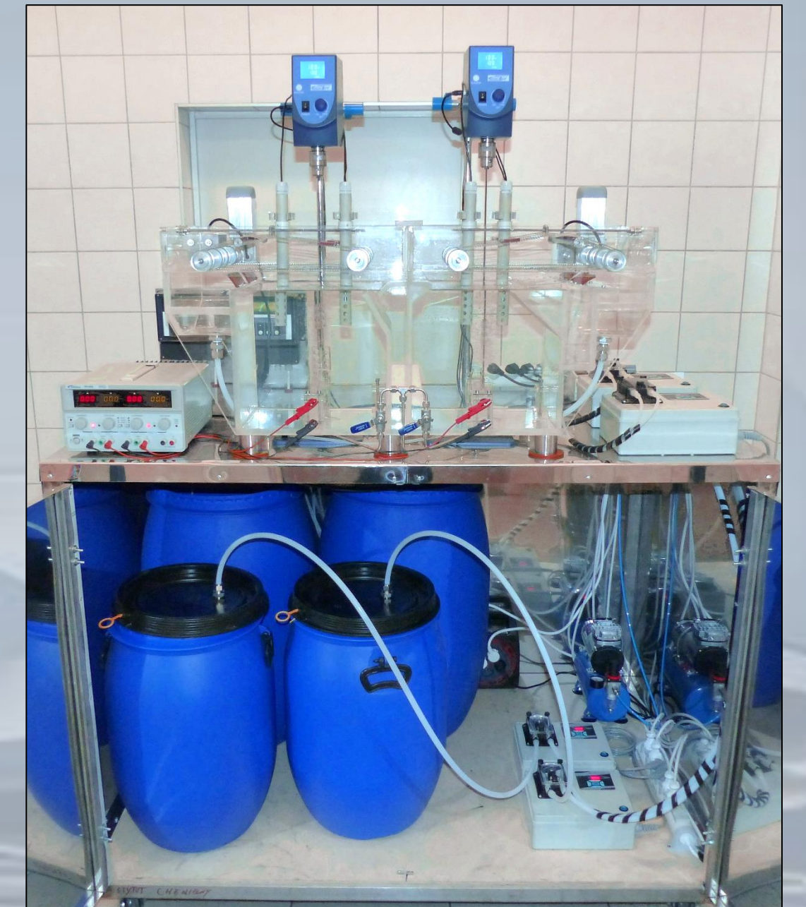
Figure 1: Pilot scale reactor for continuous electrocoagulation process
