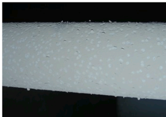
Fig. 3. Picture of F_C_01 filters with only a few patches of removed filter cake.
