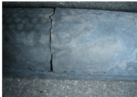
Fig. 4. Mechanical failure of filter membrane (F_M_01).
