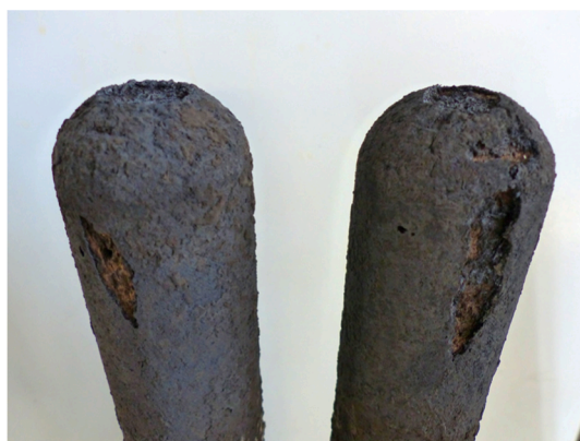
Fig. 13. Picture of ceramic filters F_C_01 after 1.5 years of testing in the 2nd gen. filter.
