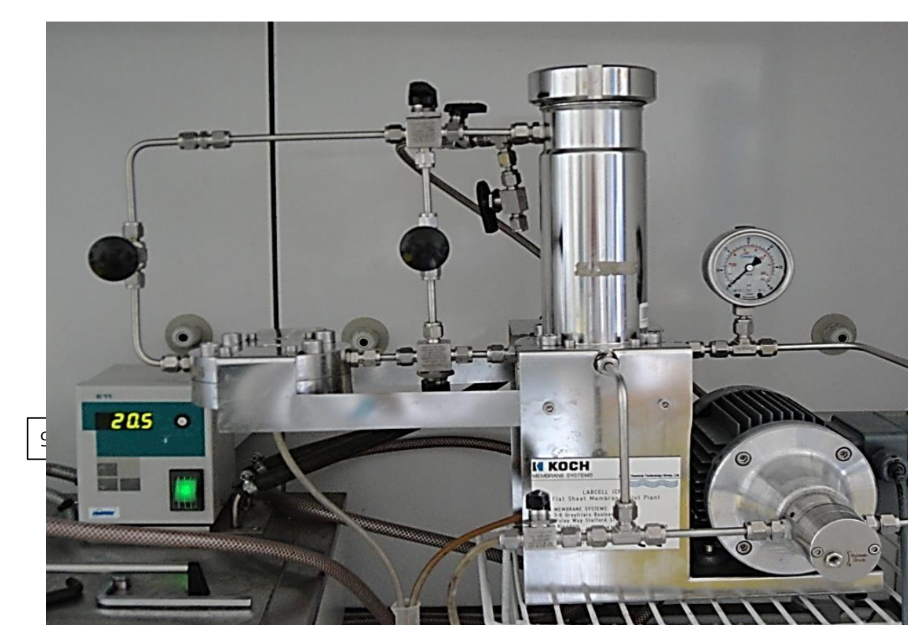
Fig. 1. KMS Cell CF1 lab-scale membrane filtration unit
