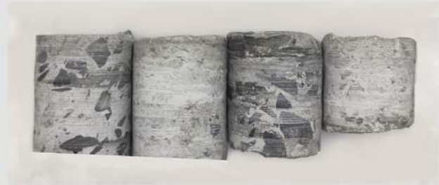
Mine shaft sample used to develop methodology of compressive strength changes during time
